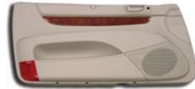
FlexForm compacts 22 layers of offset material into a 15-mm substrate weighing 1,600 g/m 2 for the Chrysler Sebring convertible's door panels. The part has a 4-in. draw.
