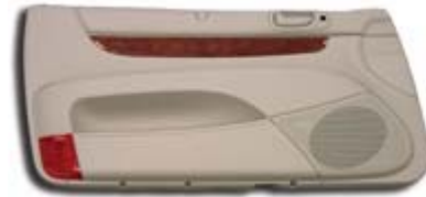
FlexForm compacts 22 layers of offset material into a 15-mm substrate weighing 1,600 g/m 2 for the Chrysler Sebring convertible's door panels. The part has a 4-in. draw.
